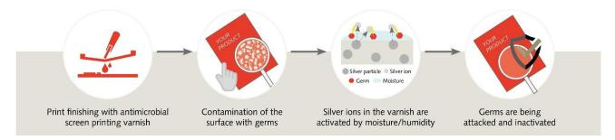
The active agent released on the coated surfaced eradicates over 99.99 per cent of germs, with a germ reduction value of > 3 log levels tested according to JIS Z 2801-2010 NORM.
